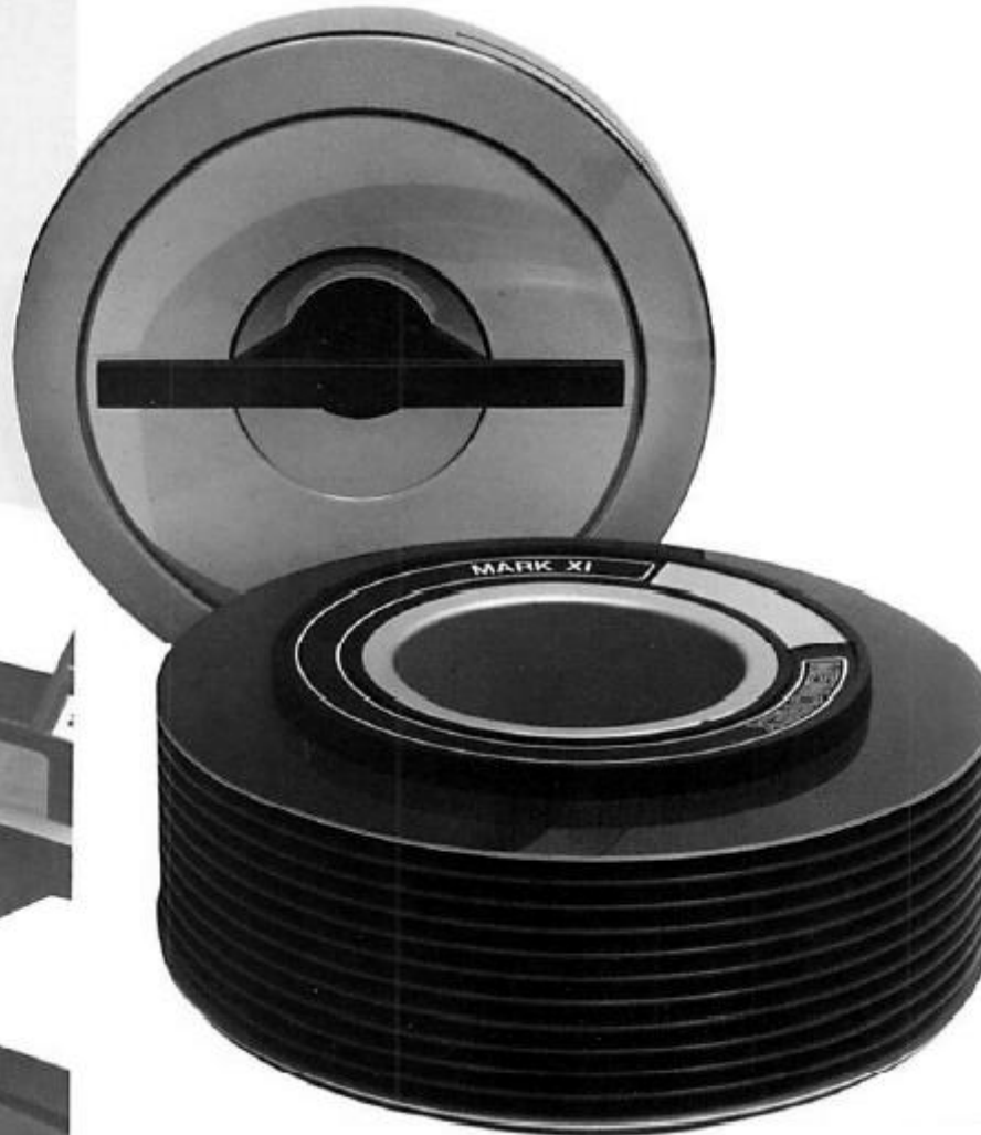
Memorex Mark XI Disc Pack 1970's about 200 Mb (IBM3336-11) PDP-10
