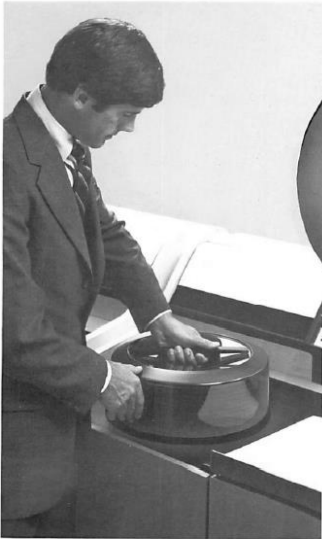
Memorex Mark XI Disc Pack 1970's about 200 Mb (IBM3336-11) PDP-10
