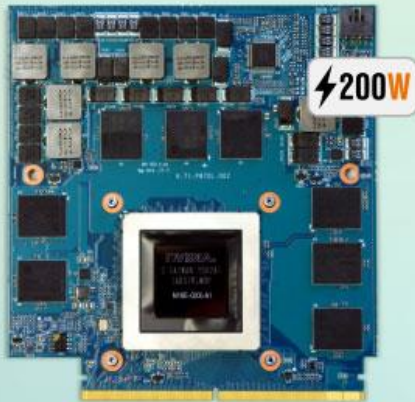
GTX 980 MXM 3.0 GPU 102.6x115mm
