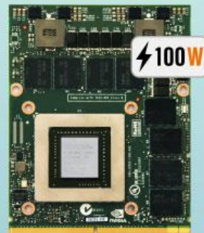
Quadro K5100M MXM 3.0b GPU 82x105mm
