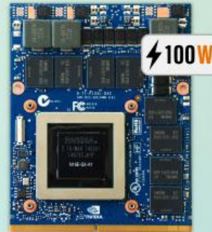
GTX 980M MXM 3.0b GPU 82x105mm
