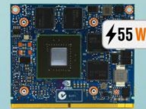
Quadro K1100M MXM 3.0a GPU 80x70mm
