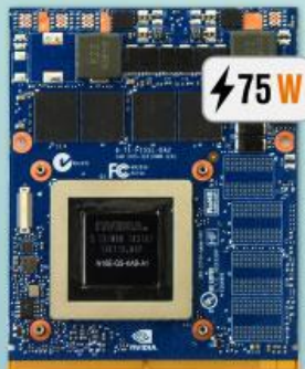
GTX 965M MXM 3.0b GPU 82x105mm
