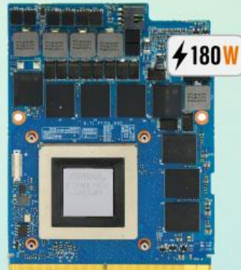
GTX 980 MXM 3.0 GPU 83x115mm
