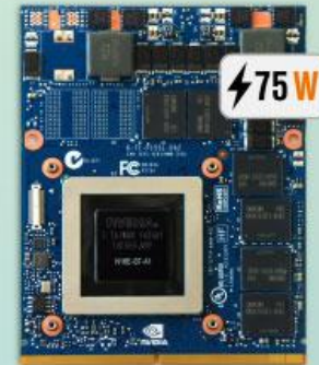
GTX 970M MXM 3.0b GPU 82x105mm
